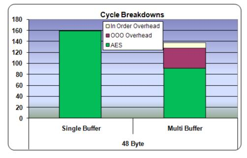
From this, we can see that even for small buffers, the out-of-order overhead is still small enough that the multi-buffer version performs better than the single-buffer version, and also that the overhead for returning buffers in order is yet smaller. As the average buffer size increases, the relative contribution of the scheduler overhead becomes much smaller.
