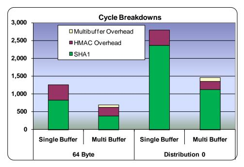
These graphs clearly show that even for small buffers, the overhead of the multi-buffer scheduler is still much smaller than the cost of computing the HMAC digest, and that the improved SHA1 performance causes the overall performance increase.
