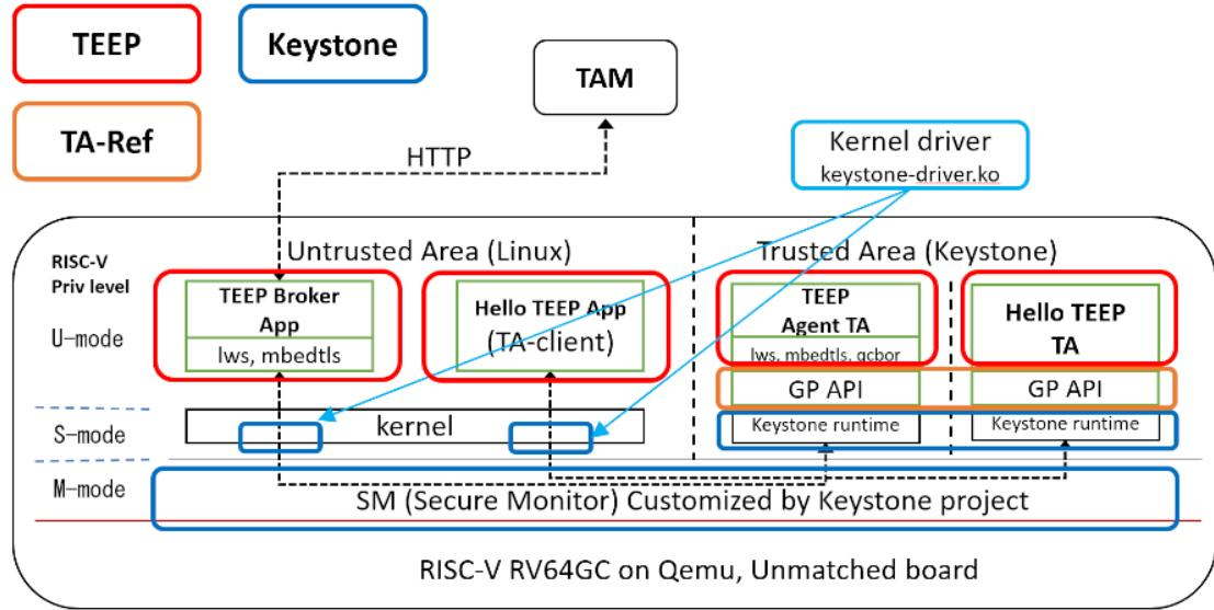
The TEEP-Device is implemented on top of the TA-Ref with TEE provided by the Keystone project on RISC-V RV64GC CPU. Each TA in the Trusted Area is protected with Physical memory protection (PMP) which is enabled by RISC-V hardware.
