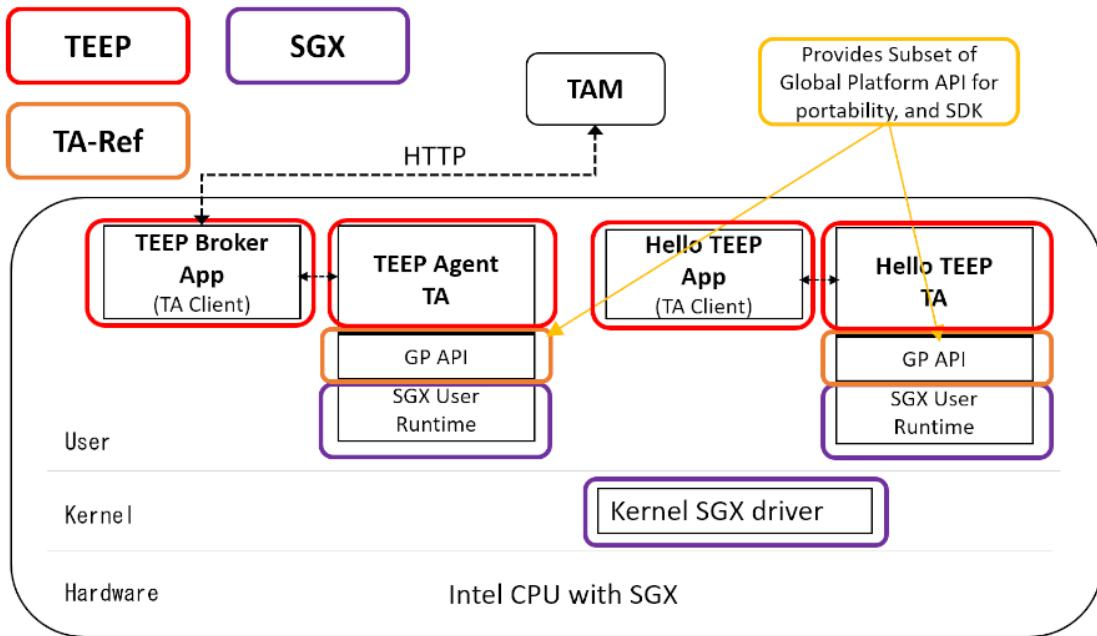
The diagram is the ideal implementation of TEEP-Device on SGX. The current TEEP-Device is not utilizing SGX libraries and the SGX enabled CPU which provides SGX capability with SGX SDK. The TEEP-Device is built and executed as a regular user space application at the moment, and enabling the SGX capability is a future activity.
