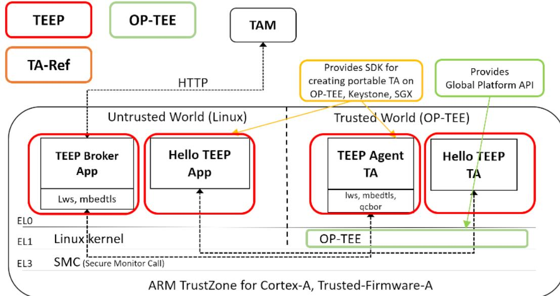
It is on OP-TEE but highly utilizes the programming environment provided by TA-Ref to simplify the TEEP-Device to be able to build and function on other CPUs with the single source code of TEEP-Agent and Hello-TEEP-TA. They both are using the subset of Global Platform API.
