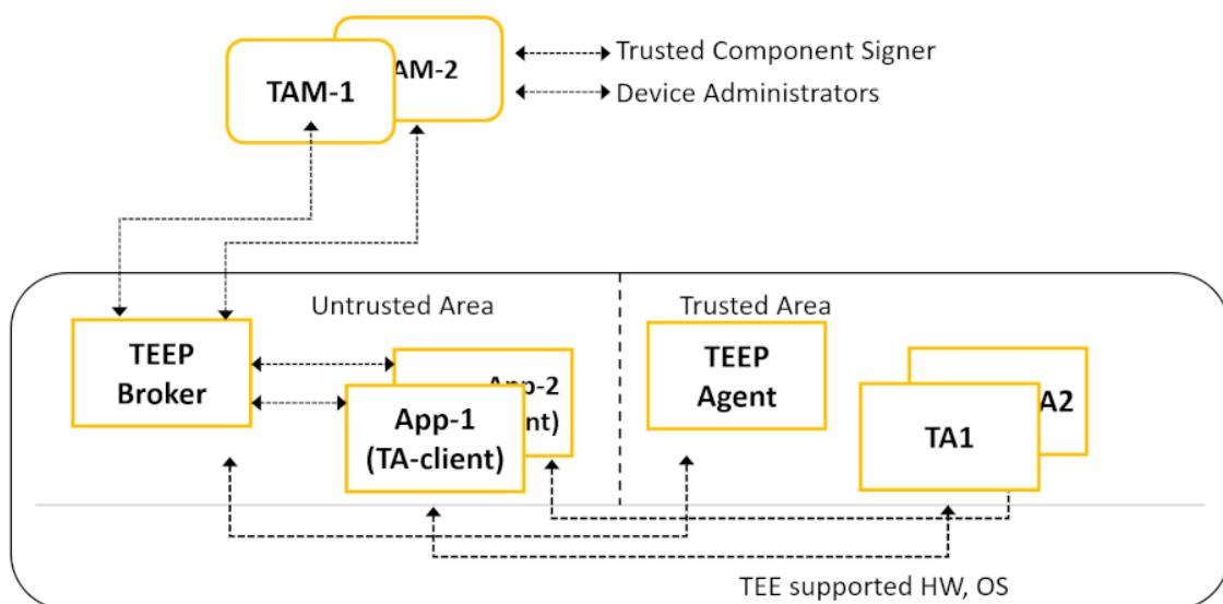
The TEEP-Device is an implementation for defining the draft of Trusted Execution Environment Provisioning (TEEP) Protocol at the Internet Engineering Task Force (IETF). The chart above is a simplified diagram of components described in the TEEP Protocol and TEEP Architecture drafts. The TEEP Protocol on the TEEP-Device uses HTTP packets defined by HTTP Transport for Trusted Execution Environment Provisioning.
