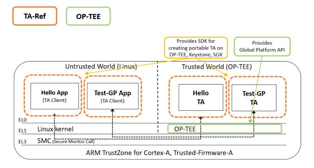
It is on OP-TEE and highly utilizing the programming environment provided by TA-Ref to simplify developing of Trusted Applications to be able to build and function on other CPUs with the single source code.
