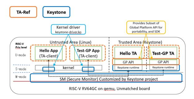
TA-Ref provides a portable TEE programming environment over the Keystone project on RISC-V RV64GC CPU. Each TA in the Trusted Aria is protected with Physical memory protection (PMP) which is enabled by RISC-V hardware.
