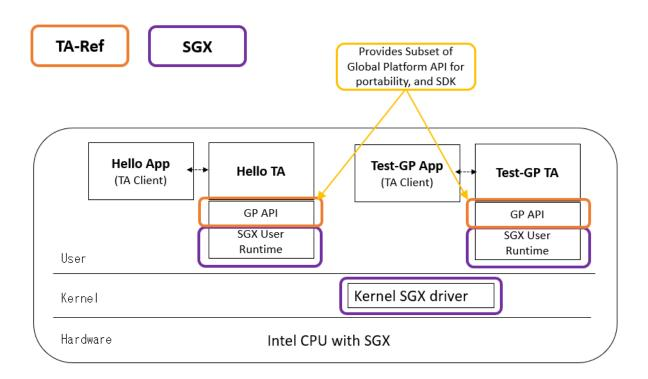
The diagram shows implementation of TA-Ref and Trusted Applications on SGX. Unlike ARM Cortex-A or RISC-V, the TEE security level is implemented vertically in the user space. The TA-Ref provides the same programming environment of ARM Cortex-A or RISC-V on Intel with the capability subset of Global Platform TEE Internal APIs.
